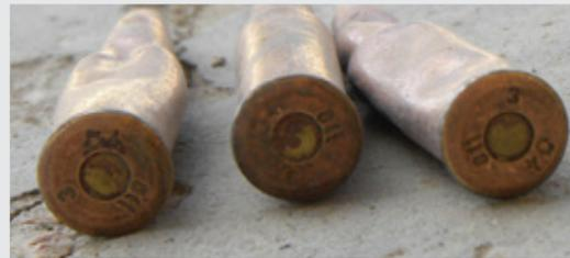
**Sudanese 7.62 x 54R mm cartridges, manufactured in 2011, with headstamps 3\_54\_011**
