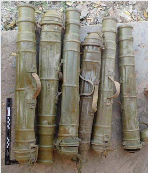
**Tubes containing 82 mm ammunition for B-10 recoilless rifles, visibly damaged, consistent with lateral impact as a result of airdropping**
