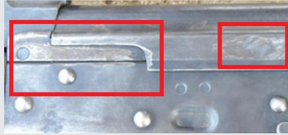
**Type 56-1 with marks removed by grinding**
