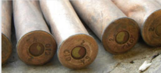
**Sudanese 7.62 x 54R mm cartridges, manufactured in 2012, with headstamps 2\_54\_012**
