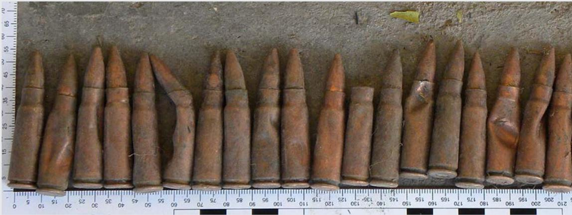
**7.62 x 39 mm ammunition, visibly damaged, consistent with sudden impact as a result of airdropping**
