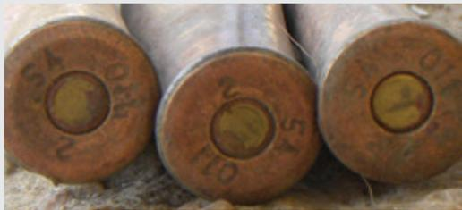
**Sudanese 7.6 x 54R mm cartridges, manufactured in 2011, with headstamps 2\_54\_011**
