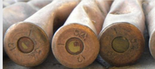
**Sudanese 7.62 x 54R mm cartridges, manufactured in 2012, with headstamps 1\_54\_12**
