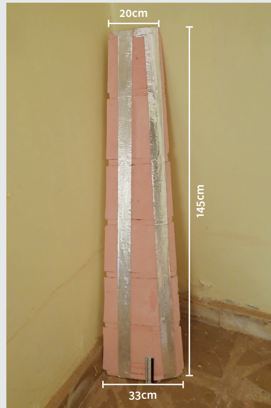
A wing in extruded polystyrene foam (used in insulation boards)
