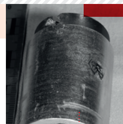
Modified North Korean submunition adapted to be attached to an FPV UAV, documented by CAR in 2025.
