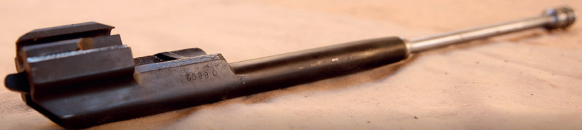
Bolt carrier from a Kbk-AKMS assault rifle documented in Bilma, Niger.
