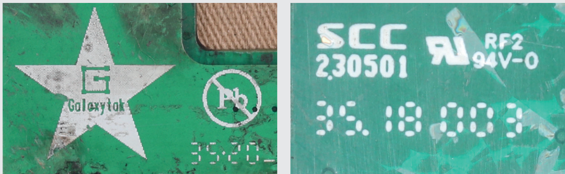
Figure 7 Printed circuit boards manufactured by Chinese companies Galaxytak-pcb Co., Ltd. (left) and Shennan Circuits Co., Ltd. (right) from two different strikes on 24 February and 1 April 2022.
