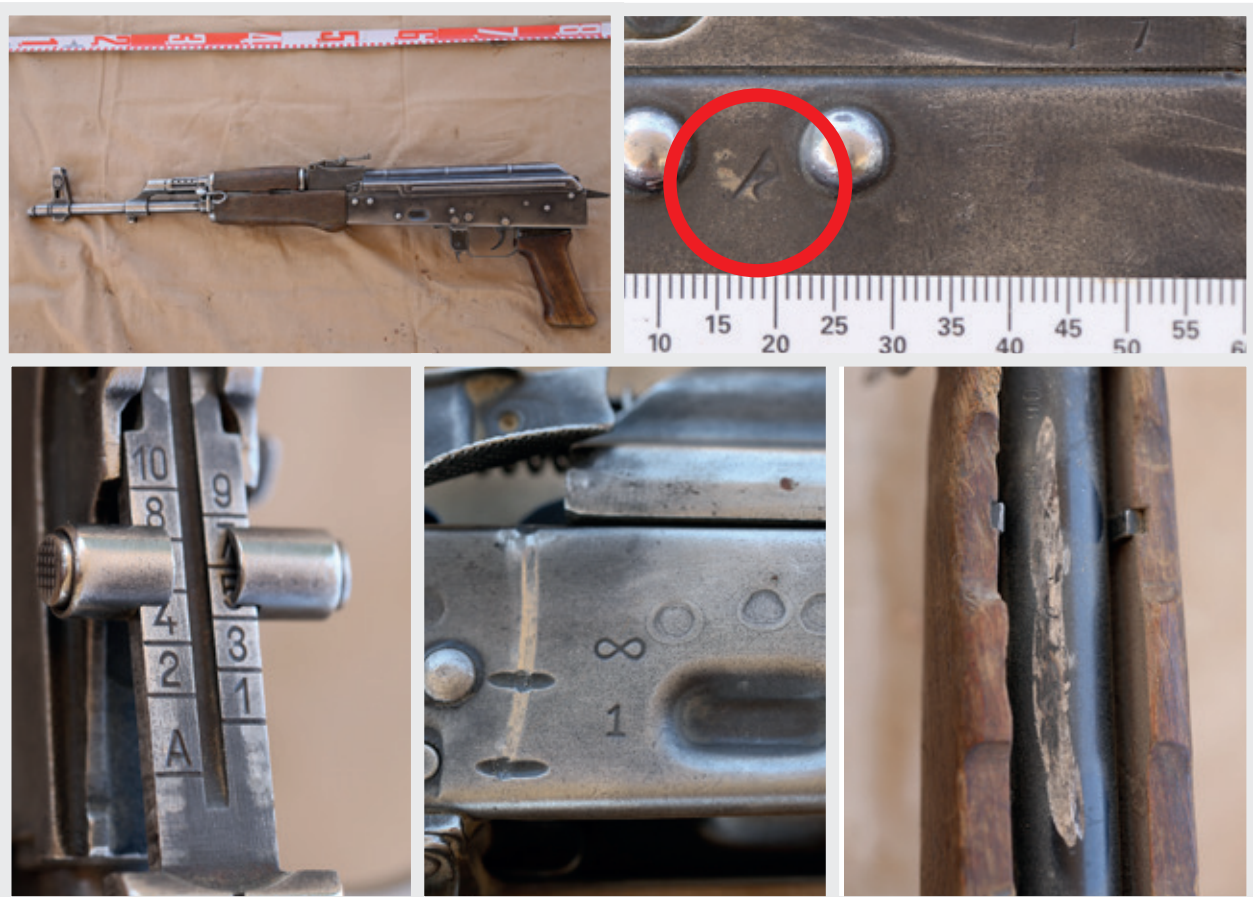
An AK-63F-pattern rifle with markings reflective of Hungarian manufacture, an obliterated serial number, and an Iraqi arsenal mark (circled), documented in Diffa in 2019
