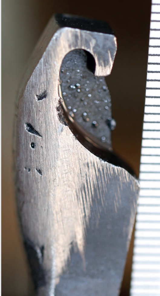
Figure 6 Hammer (left-hand side), displaying tool marks
