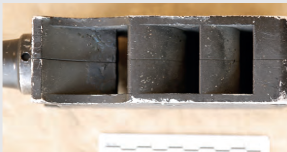
Figures 20 and 21 Profile of the muzzle brake with vents
