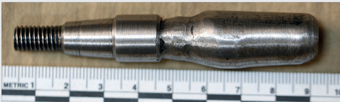
Figure 26 Replacement bolt handle
