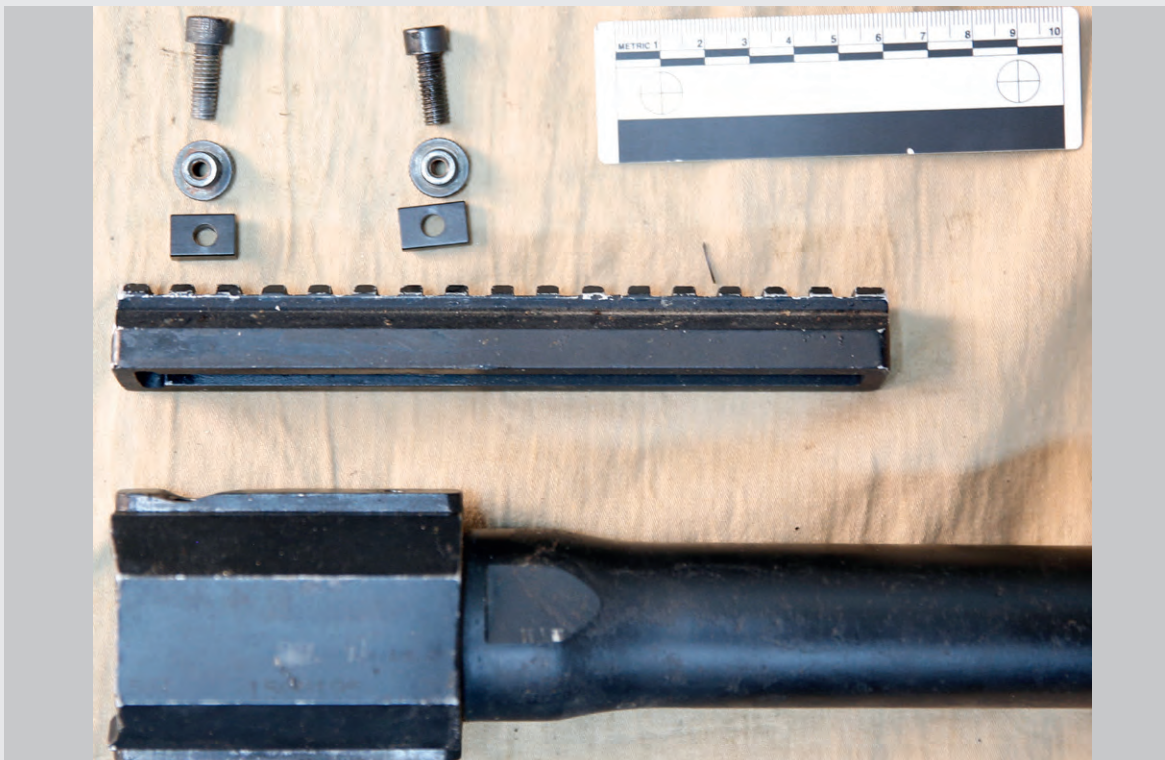
Figure 17 Scope rail sub-assembly with the two screws that are used to fasten it atop the barrel and two fasteners for the optics
