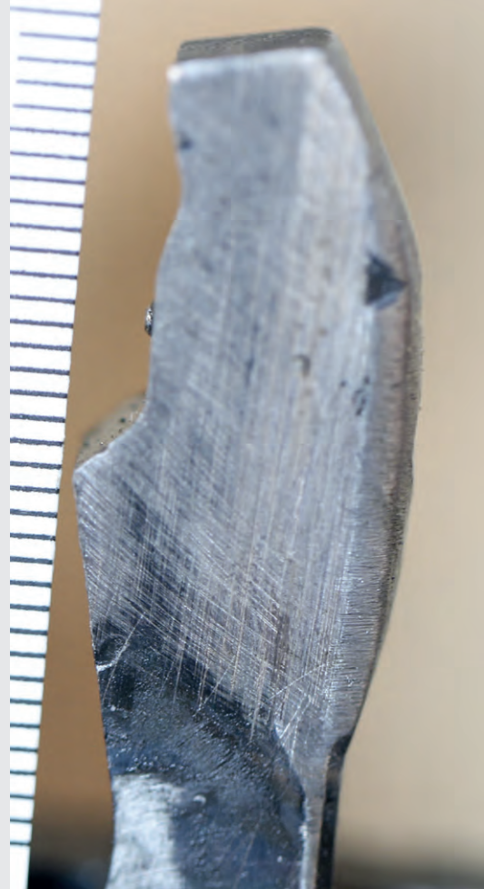
Figure 7 Hammer (right-hand side), displaying tool marks
