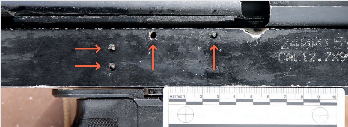
Figure 4 Three of four pins designed to retain the trigger group within the housing (see arrows)
