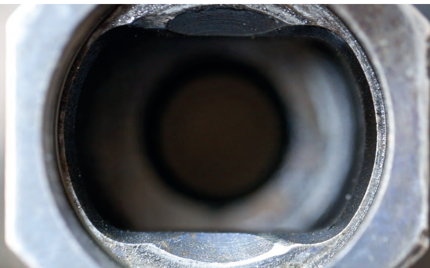
Detail of an AM-50 chamber, showing the locking lugs.
