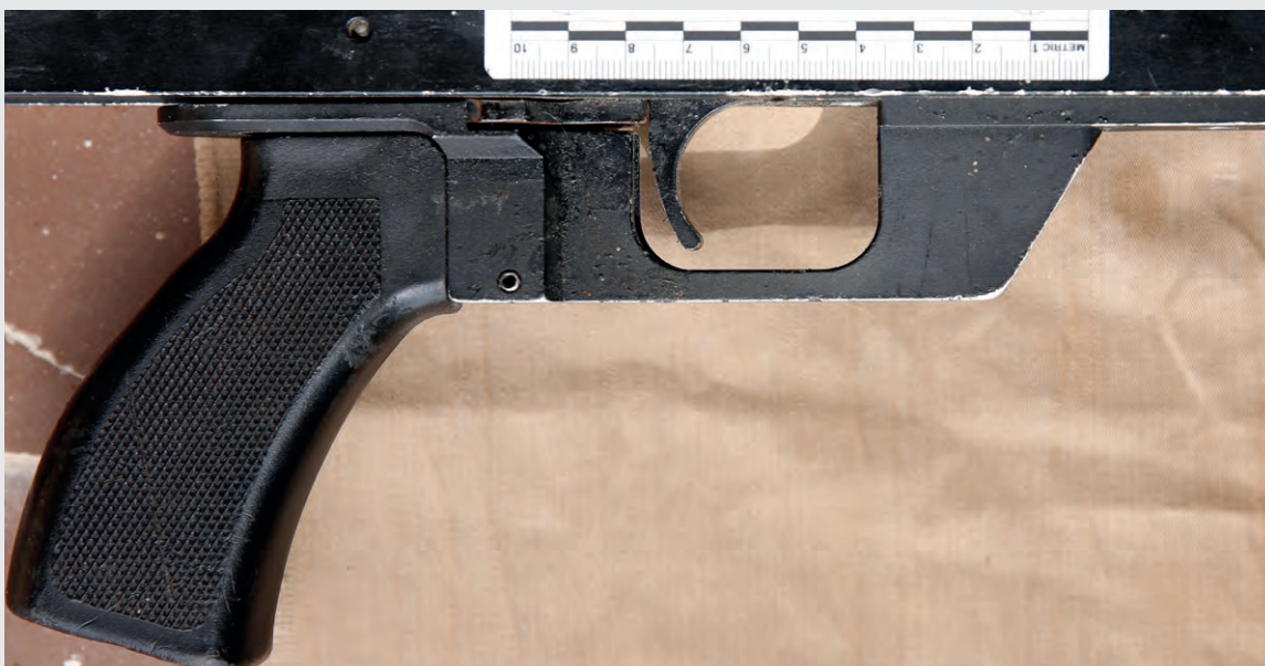
Figure 5 Trigger guard, trigger, safety, and pistol grip
