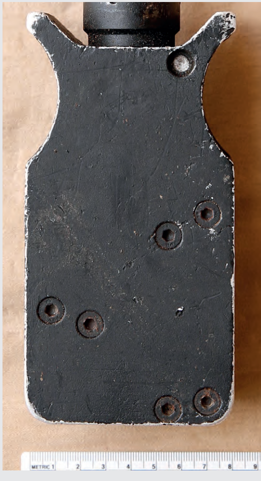
Figure 18 Underside of the muzzle brake with six hex-head cap screws (distributed in three pairs for each vent) and an additional headless screw
