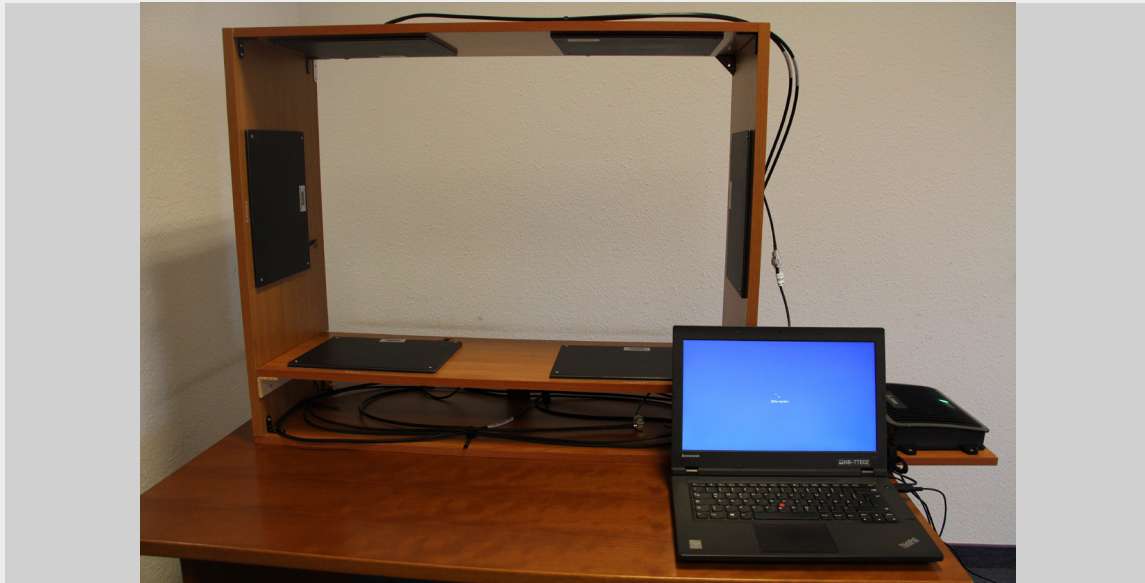
Figure 24 UHF test gate A
