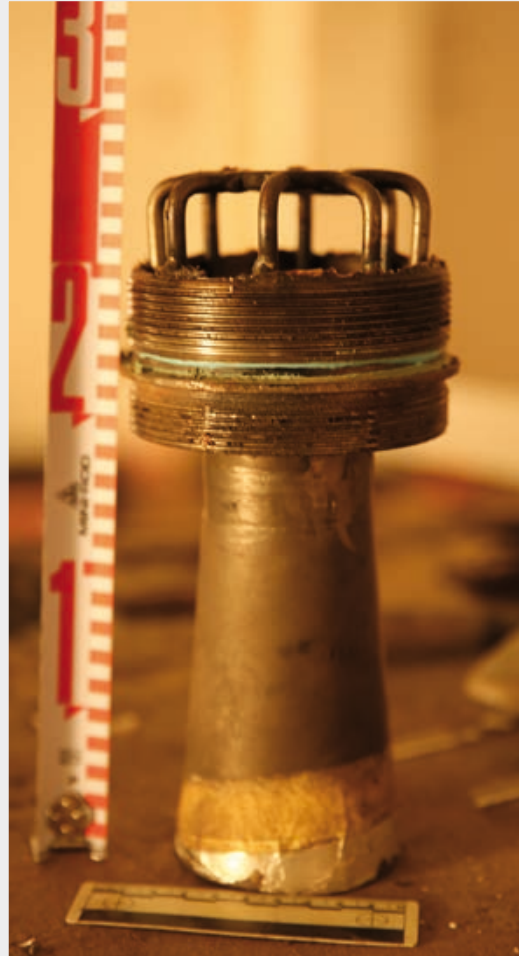
Image 20 115 mm rocket nozzle Qaraqosh, November 2016
