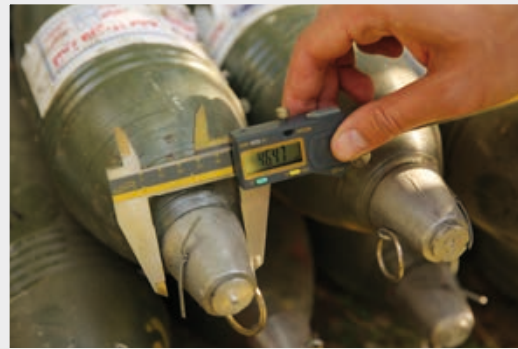
Image 7 A point-detonating fuse for a 120 mm mortar round manufactured by IS forces Gogjali, Mosul, November 2016
