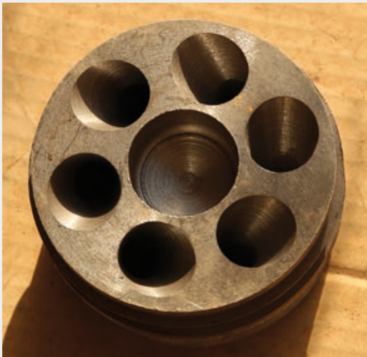
Image 19 Short rocket exhausts Qaraqosh, November 2016
