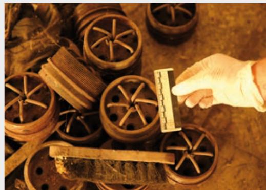
Image 21 115 mm rocket base, inside view Qaraqosh, November 2016
