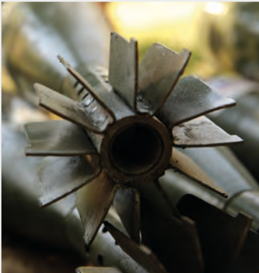
Image 6 A 120 mm mortar round fin assembly manufactured by IS forces Gogjali, Mosul, November 2016
