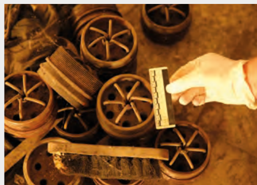
Image 21 115 mm rocket base, inside view Qaraqosh, November 2016
